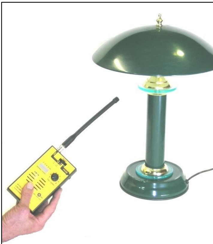
(FIG. 4) ANTENNA SCAN OF A SUSPECT NOISE SOURCE
